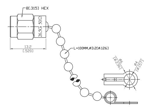
2W average power from -55°C to 70°C linearly derated to 1 Watt at 165°C
