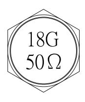
2W average power from -55°C to +70°C linearly derated to 1 Watt at 165°C
