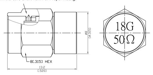
2Watt Average Power From -55°C/+70°C Lineary Derated to 1Watt At 165°C
