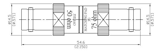
Power Rating: 0.5W Continuous Operating Temp: -30°C / +70°C
