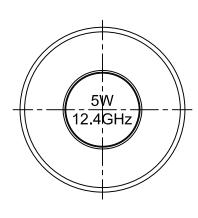
5W average power from -55°C to +70°C linearly derated to 1.5 Watt at 165°C
