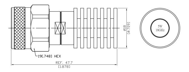
5W average power from -55°C to +70°C linearly derated to 1.5W at 165°C
