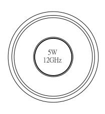
5W average power from -55°C to +70°C linearly derated to 1.5W at 165°C
