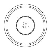
5W average power from -55°C to +70°C linearly derated to 1.5W at 165°C
