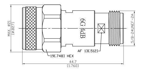
Nominal impedance:  $50\Omega\pm0.25\Omega$  over operating temperature range.
