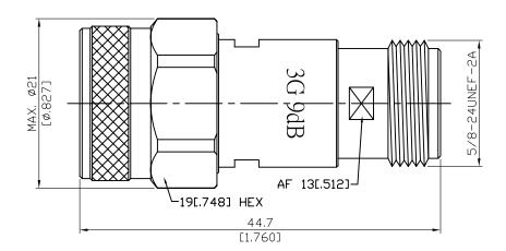
Nominal impedance:  $50\Omega \pm 0.25\Omega$  over operating temperature range.
