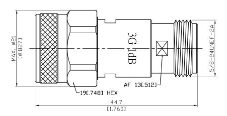
Nominal impedance:  $50\Omega \pm 0.25\Omega$  over operating temperature range.
