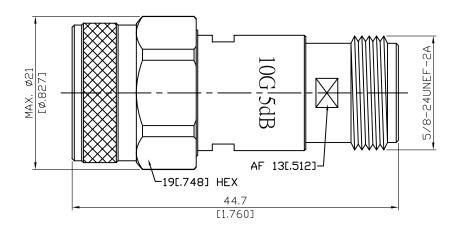
Nominal impedance:  $50\Omega\pm0.25\Omega$  over operating temperature range. Operating temperature range: -50 degrees Celcius to +80 degrees Celcius.
