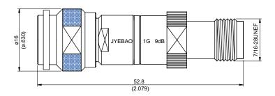
Nominal impedance:  $50\Omega$ +/-0.25 $\Omega$  over operating temperature range. Operating temperature range: -50 degrees Celcius to +80 degrees Celcius.
