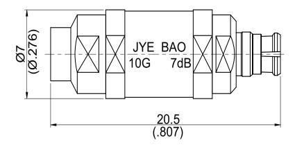
Nominal impedance:  $50\Omega$ +/-0.25 $\Omega$  over operating temperature range. Operating temperature range: -50 degrees Celcius to +80 degrees Celcius.
