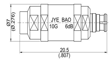
Nominal impedance:  $50\Omega$ +/-0.25 $\Omega$  over operating temperature range. Operating temperature range: -50 degrees Celcius to +80 degrees Celcius.
