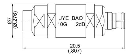
Nominal impedance:  $50\Omega$ +/-0.25 $\Omega$  over operating temperature range. Operating temperature range: -50 degrees Celcius to +80 degrees Celcius.
