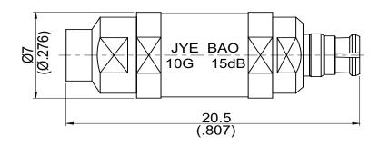
Nominal impedance:  $50\Omega$ +/-0.25 $\Omega$  over operating temperature range. Operating temperature range: -50 degrees Celcius to +80 degrees Celcius.
