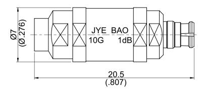
Nominal impedance:  $50\Omega$ +/-0.25 $\Omega$  over operating temperature range. Operating temperature range: -50 degrees Celcius to +80 degrees Celcius.
