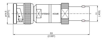
Nominal impedance:  $50\Omega + /-0.25\Omega$  over operating temperature range.
