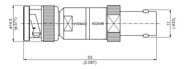
Nominal impedance:  $50\Omega \text{+/-}0.25\Omega$  over operating temperature range.
