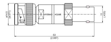
Nominal impedance:  $50\Omega \text{+/-}0.25\Omega$  over operating temperature range.
