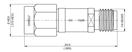
Nominal impedance:  $50\Omega+/-0.25\Omega$  over operating temperature range. Operating temperature range: -50 degrees Celcius to +80 degrees Celcius.
