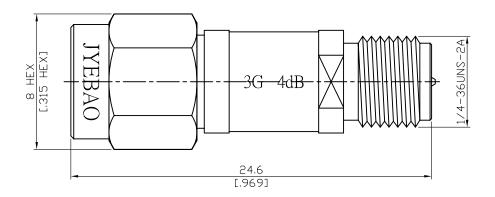
Nominal impedance:  $50\Omega\pm0.25\Omega$  over operating temperature range.
