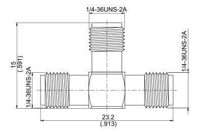
NOTE: T-adaptor is a non-matched 3 dB divider for low frequency applications. VSWR  $\geq$  2.0 when terminated 50  $\Omega$ .
