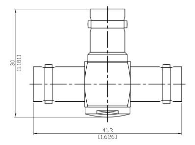
Dielectric withstanding voltage (at sea level): 5000 V rms Working Voltage (at sea level): 1600 V rms
