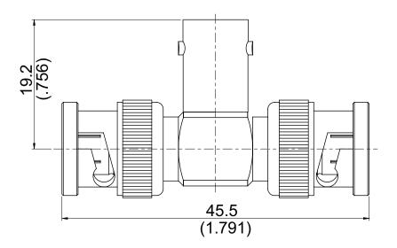
NOTE: 50  $\Omega$  nominal impedance. This connector is a non-matched 3 dB divider for low frequency applications. VSWR  $\geq$  2.0 when terminated 50  $\Omega$ .
