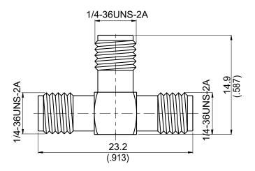
NOTE: 50  $\Omega$  nominal impedance. This connector is a non-matched 3 dB divider for low frequency applications. VSWR  $\geq$  2.0 when terminated 50  $\Omega$ .
