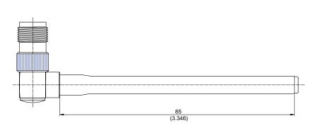
1.8 GHz TNC Jack Right Angle Dipole Antenna
