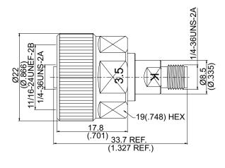
Note:Ruggedized 3.5 jack to be mounted directly on vector network analyzer.
