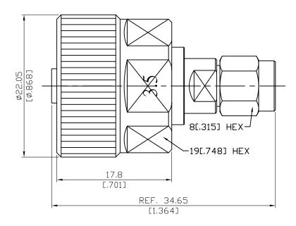
Note:Ruggedized 3.5 jack to be mounted directly on vector network analyzer.
