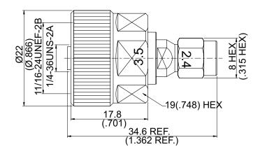
Note:Ruggedized 3.5 jack to be mounted directly on vector network analyzer.
