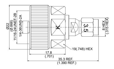
Note:Ruggedized K jack to be mounted directly on vector network analyzer.
