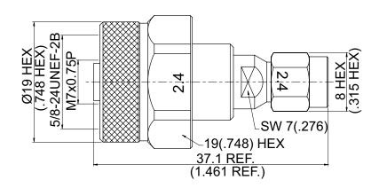
Note:Ruggedized 2.4 jack to be mounted directly on vector network analyzer.
