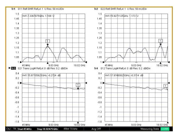
Note: S11/S12/S21/S22 plots shown represent IL and VSWR of two adaptors tested. To extract IL of a single adaptor divide IL measured by two.
