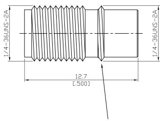
\*SMA Jack Snap On Design With Short Thread Ensuring Excellent Mating Reliability. \*Snap On And Give One Turn For Proper Mating
