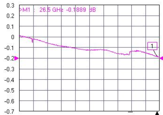
Tr4 S21 Trans LogM RefLvl: -0.2 dB Res: 0.1 dB/Div
