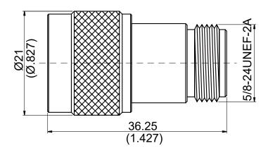
NOTE: N Plug Snap On Adaptor Without Locking Mechanism.
