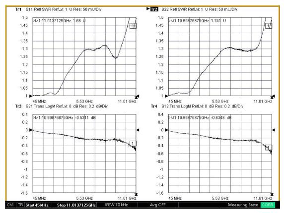
Note: S11/S12/S21/S22 plots shown represent IL and VSWR of two adaptors tested. To extract IL of a single adaptor divide IL measured by two.
