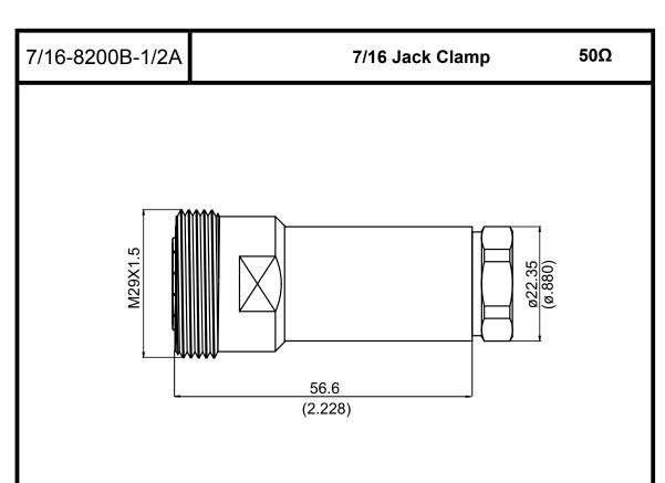
NOTE: (1) FOR 1/2 " FOAM DIELECTRIC CABLE. (2) LOW INTERMODULATION DESIGN.
