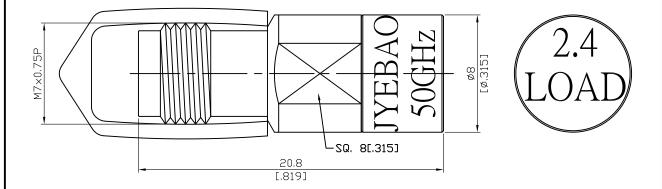
1 W Average Power From -40°C to 70°C Linearly Derated To 0.7 Watt at 105°C
