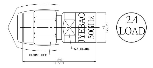
1 W Average Power From -40°C to 70°C Linearly Derated To 0.7 Watt at 105°C
